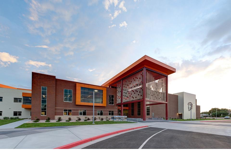
Front entry canopy designed using proportions of the Golden Section, infilled with suspended metal panels to create unique and constantly changing patterns with the sun's movement.
