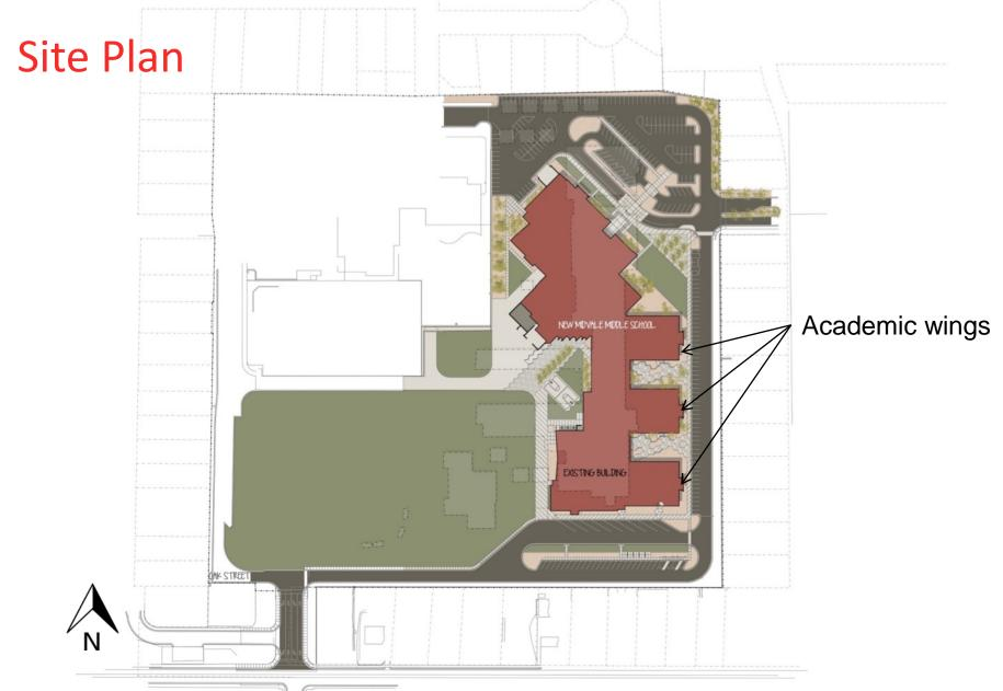
Academic wings are oriented along an east/west axis, allowing only north or south light (which is controlled by shading devices) to enter the classrooms.
