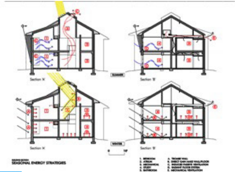
Navajo Prep – Passive solar and natural ventilation
