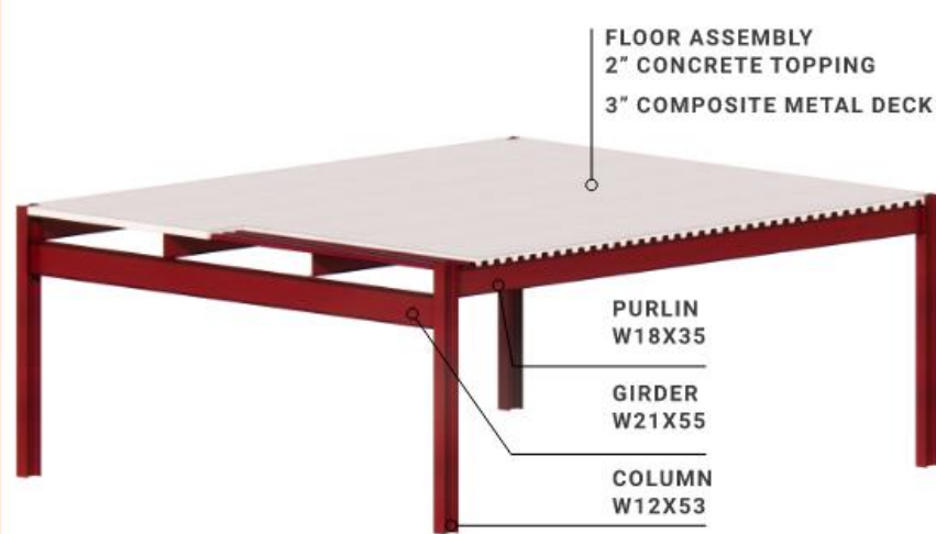
Steel Structural Bay
