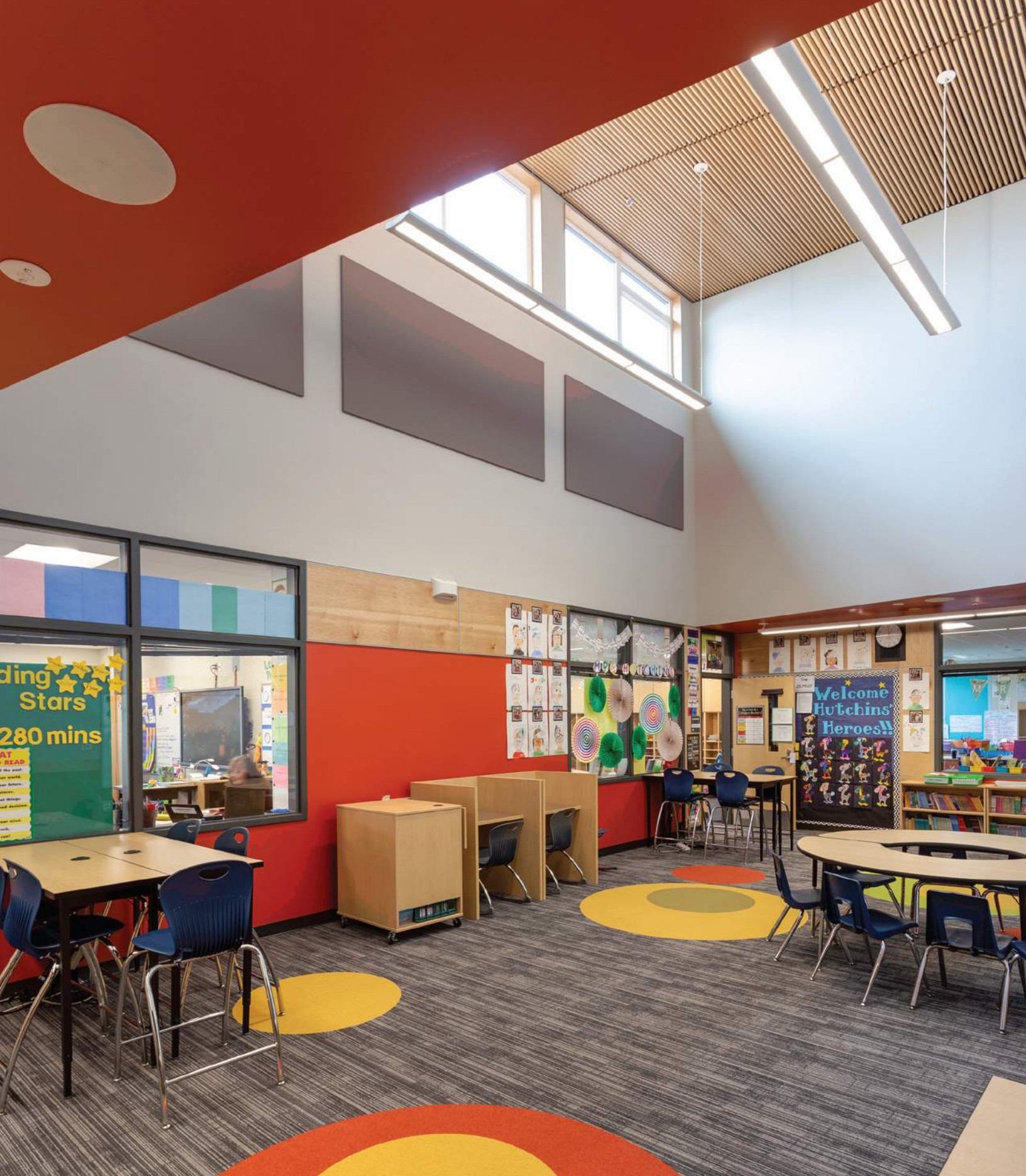
Above: The upper floor shared learning area fill with natural light. Flexible furniture allows the spaces to be used in small groups or for individual study. The acoustical wall panels, tapered side walls and wood slat ceiling provide acoustical benefits for student learning.
