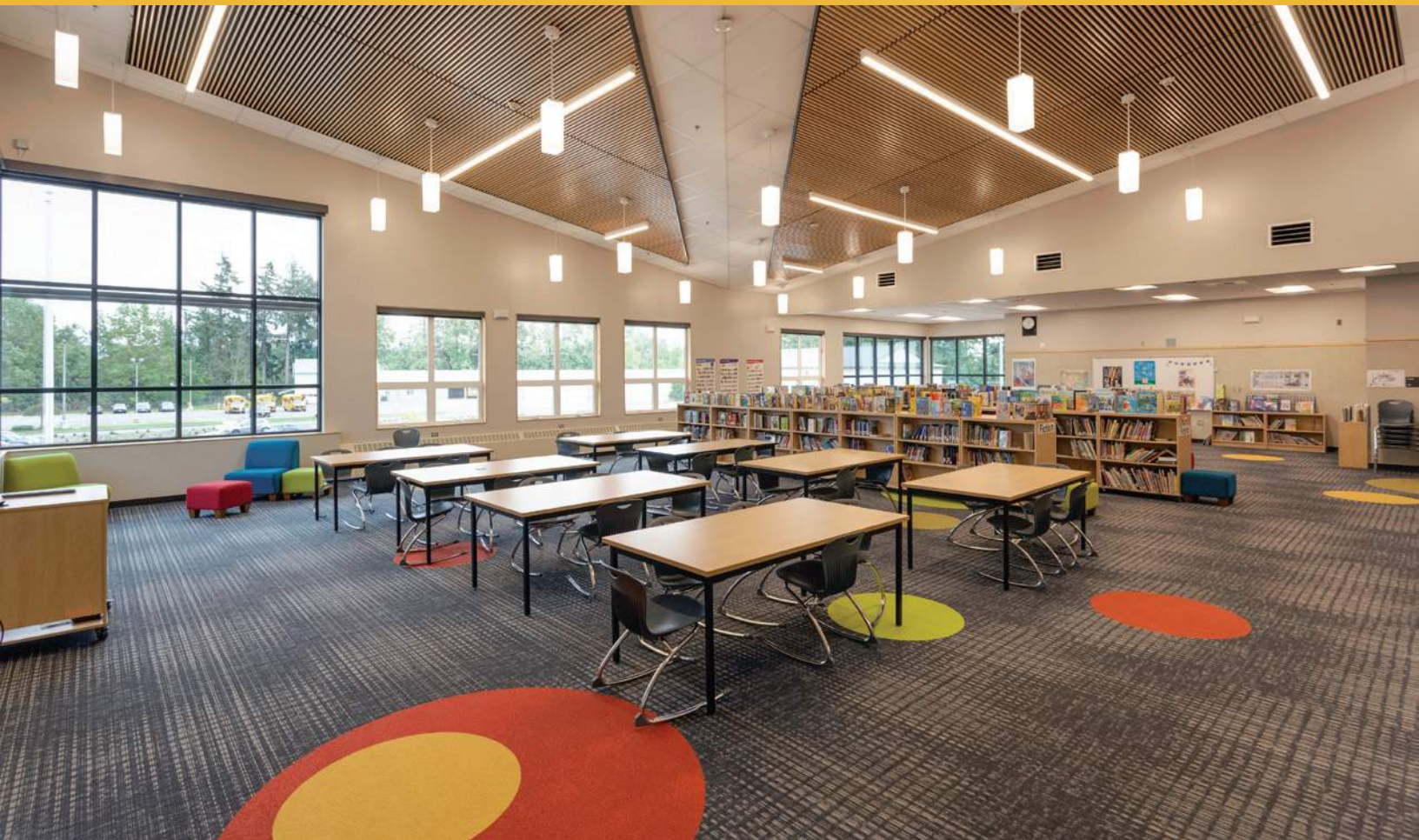
Above: Typical entry into the shared learning area with classrooms to the left and beyond. The relites and windows were designed to allow passive supervision of shared learning area and let borrowed light pass between rooms.
