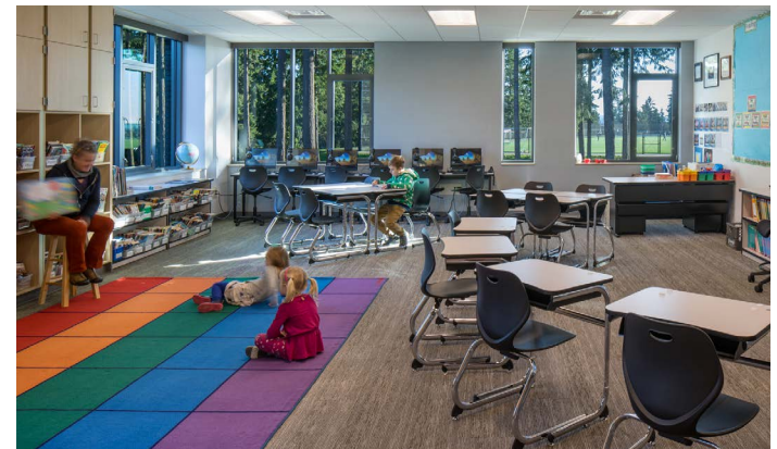
B The design of the classroom clusters allows most classrooms to have windows on two sides, maximizing daylight and providing passive energy savings.
