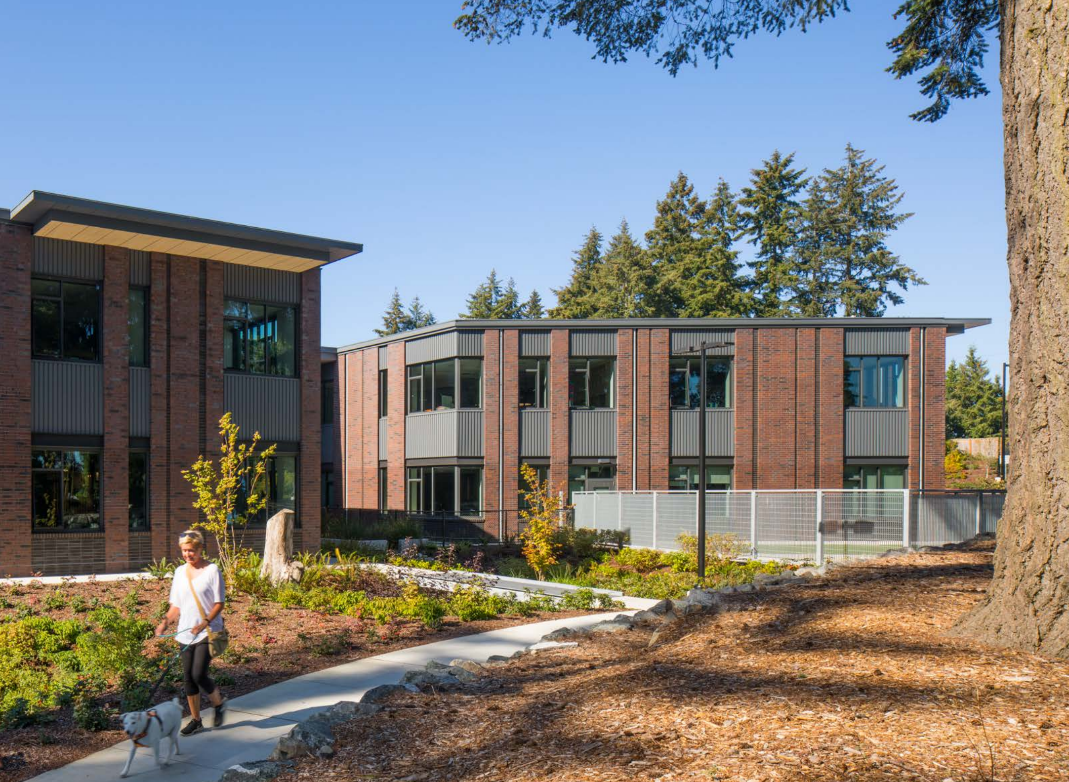
The stacked learning clusters rotate out from a central, hexagonal hallway, helping break down the overall mass of the two-story school to fit within the mostly residential neighborhood. The brick and siding colors, textures, and rhythm were chosen to evoke the character of the surrounding trees.
