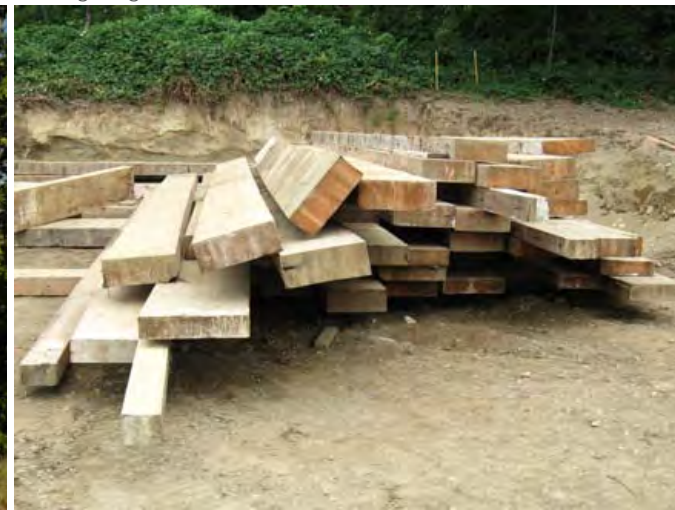
Salvaged glu-lam beams
