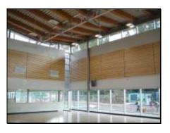
This is the studio. Wood floor, wood acoustic panels and butterfly trusses form the roof.
