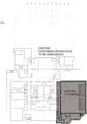
EXISTING SCHOOL DEMOLITION PLAN LOWER LEVEL
