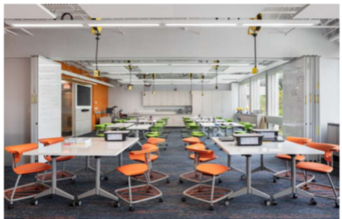
SECCM East Wing, RWU, BTGA – glazed, operable partitions turn a former block-wall corridor into a flexible, visually connected learning space.
