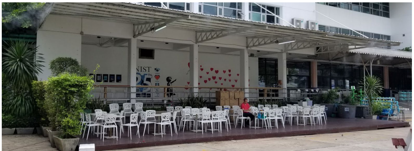
FIGURE 94. This outdoor café works because it is under a lightweight awning. Shade structures like this are easy to create and can be quickly installed to increase the amount of outdoor space that is available for use during most of the school day.
